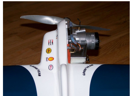
Figure 5. Be sure to install a shutoff on your Formula Unlimited. Here is a "one-shot" wire shutoff that is integrated into the motor mounting plate. The flexible
