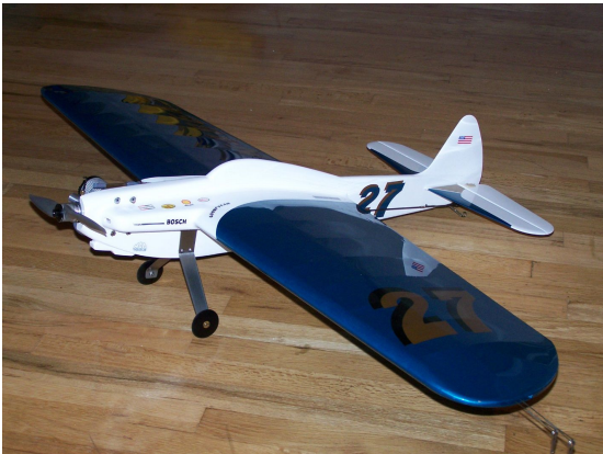
Figure 3. An early photo before the canopy was painted in and the rest of the numbers added. Of note is the titanium landing gear. This location turned out to be too far aft, and the plane would nose over when the elevator effectiveness was lost as it slowed down on the landing roll. A narrower, reduced drag set of titanium gear legs were subsequently added in a more forward location. (Photo by the author)
