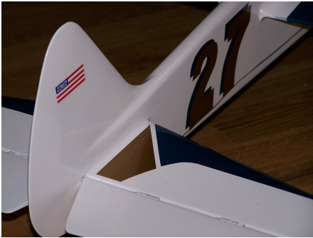
Figure 6. The tail group of the Shoestring is glassed and filleted for strength. Due to the weight of the HB engine, the extra weight of firm wood and glass in the tail improves the balance. Rare for me, I used pinned hinges on this racer. The MonoKote trim can be applied directly over the KlassKote. It takes low heat and special care to avoid lots of bubbles—and some smaller ones seem to be unavoidable. The shadowed numbers are cut out in pairs at the same time and then offset when laying them into position. (Photo by the author)
